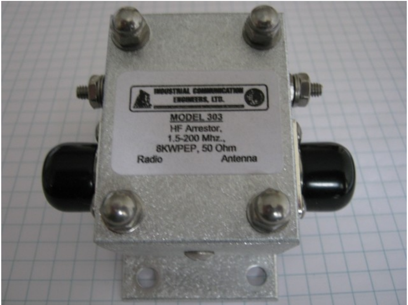
External view of ICE Model 303 surge protection device (SPD). Note the power rating! You can go ahead and buy an amp if you have this one. Thanks to KD5ZMZ for letting me photograph – and then disassemble and photograph his new toy. Photo by K5WLF.
